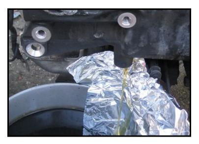
**Side note:** Before changing any oil always remove the filler plug first. The last thing you want is to drain it and then not be able to refill it. This is seldom an issue on K bikes though.
