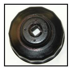
I prefer metal over plastic since the plastic ones will wear out eventually but if plastic is all you can find. The specifications for the oil wrench are a 76mm diameter with 14 flutes. AutoZone sells the "OEM" brand "B" Oil Filter Wrench - part number 25401.
