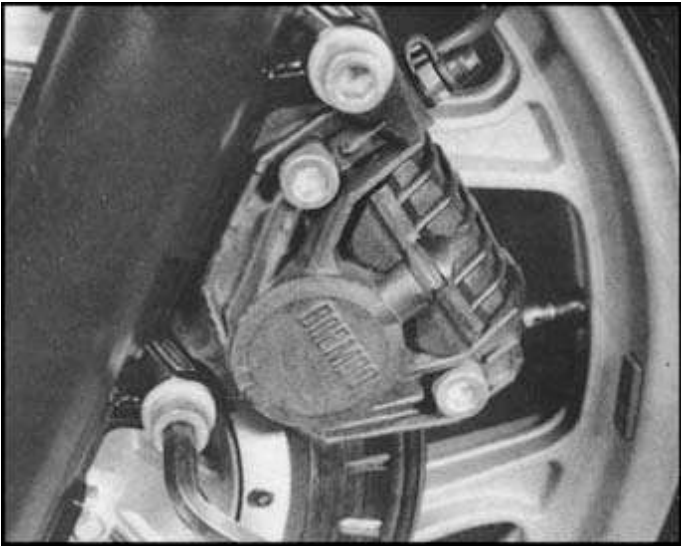
2.3 One caliper, possibly both, must be removed before the wheel can be withdrawn
