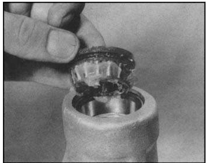
6.5 Pack bearings with specified grease on refitting
