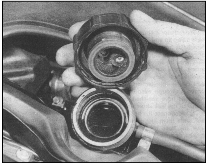
6.1 Radiator filler cap can be tested only using special equipment
