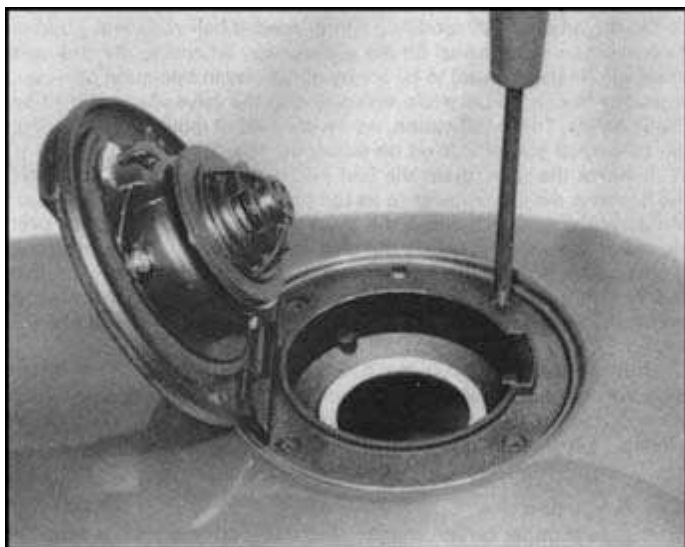
6.1 Remove retaining screws to release filler cap assembly — check gaskets carefully
