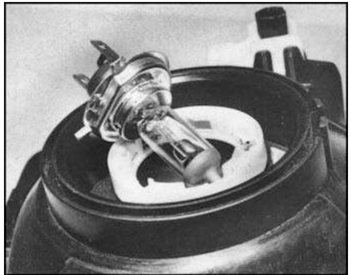
22.1b Bulb is located by offset tangs — never touch glass envelope
