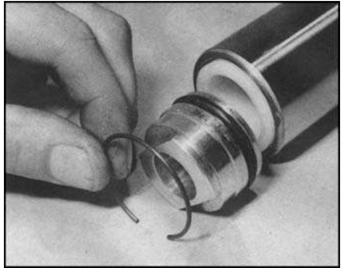
5.8c ... followed by top plug — note new sealing O-ring
