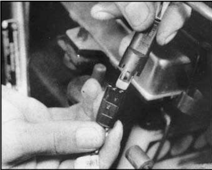
5.5b and disconnect to release tank wiring — ensure catch is fastened correctly on refitting
