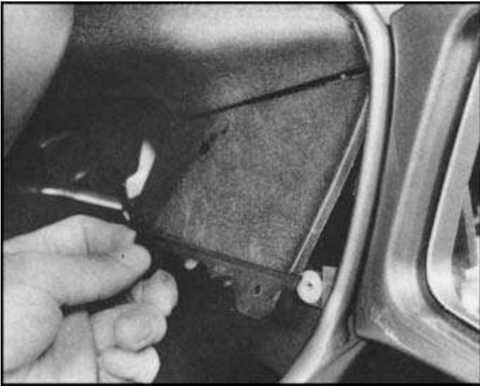
15.32a Unclip small panels from horizontal centre panel
