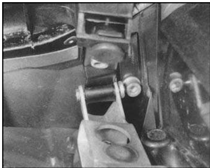
16.3 Seat mounting bracket may be unbolted if required
