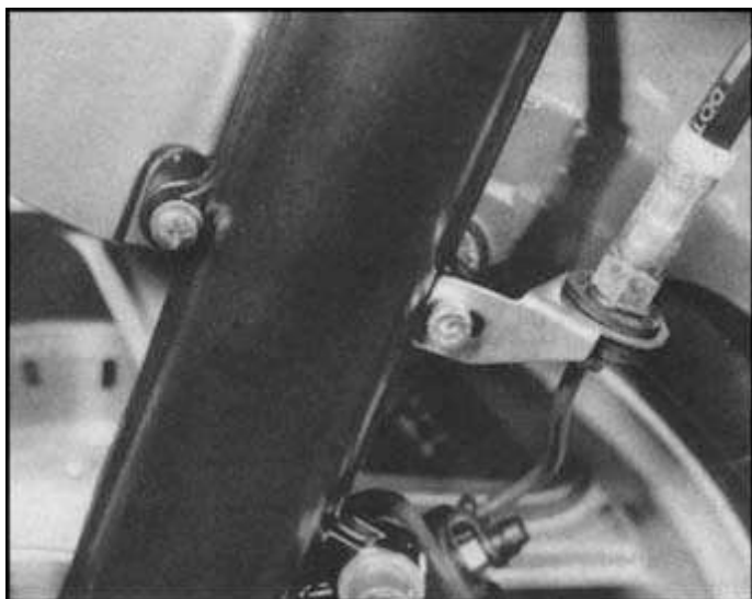
2.3 Remove front wheel, both brake calipers and hoses, and front mudguard
