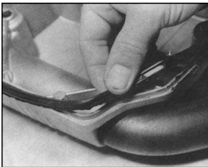
34.2b Apply smear of sealant to stick seal in cover groove
