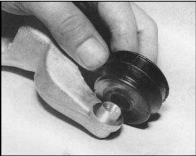
6.5 Check rubber boot for splits or tears — renew if leaking
