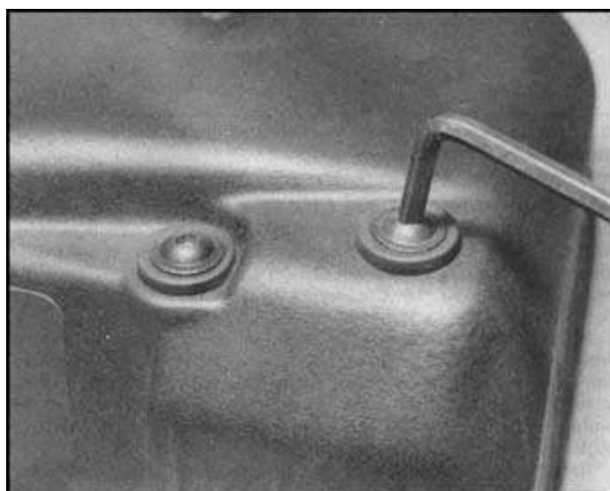
14.6a Remove two screws from top of air filter top half
