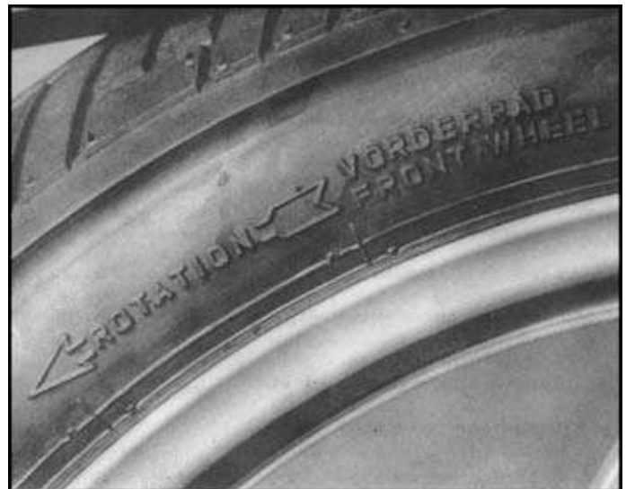
2.1 Before removing wheel, note tyre fitting mark and use to determine direction of installation
