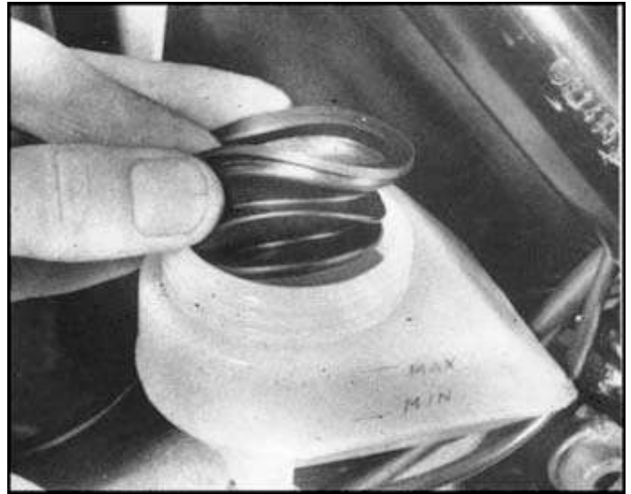
Ensure diaphragm is clean and dry before refitting
