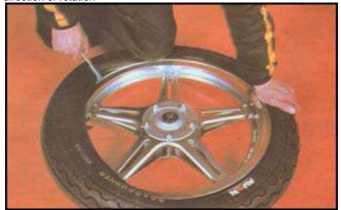
Work bead under rim towards and each side of valve using lever if necessary
