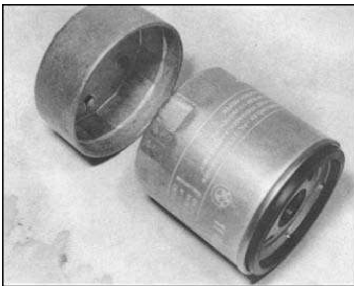
Oil filter element must be removed using special tool which engages its shaped end...
