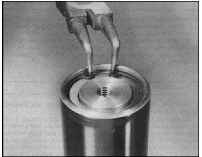
5.6c Clearance between valve housing and circlip must be eliminated using shims
