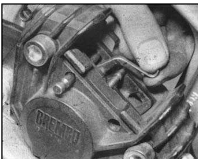
...insert first retaining pin with spring, then refit central pin, as shown...
