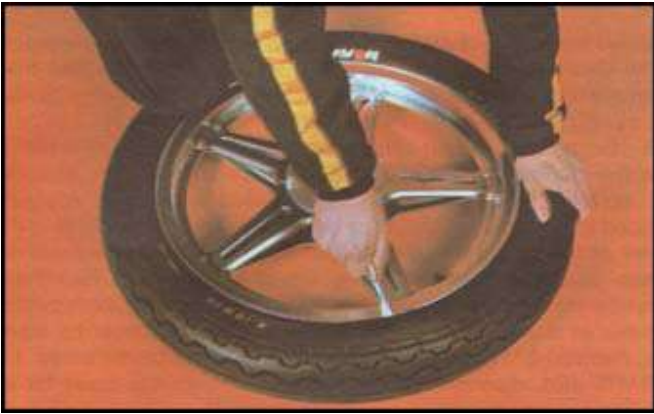
Tyre removal: Deflate tyre and insert lever in close proximity to tyre valve
