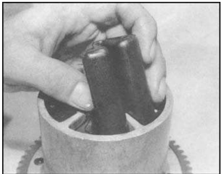
24.19a 100 models only — lubricate shock absorber rubbers to aid reassembly
