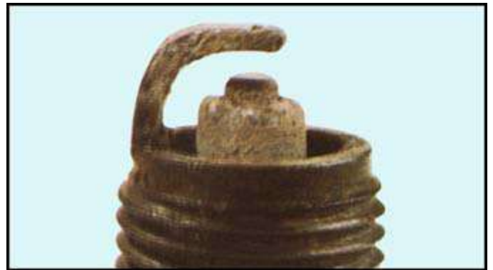
A worn spark plug not only wastes fuel but also overload the whole ignition system because the increased gap requires higher voltage to initiate the spark. This condition can also affect air pollution
