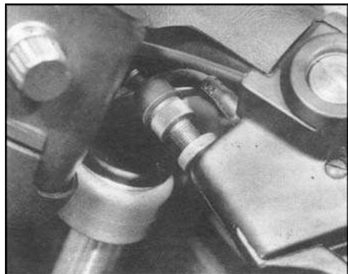
Use cable handlebar adjuster to set
