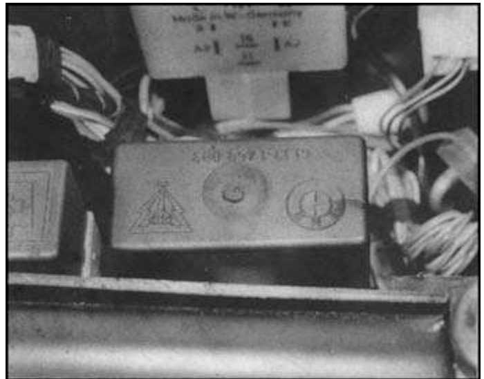
16.1 Tail lamp bulb monitor must be renewed if faulty
