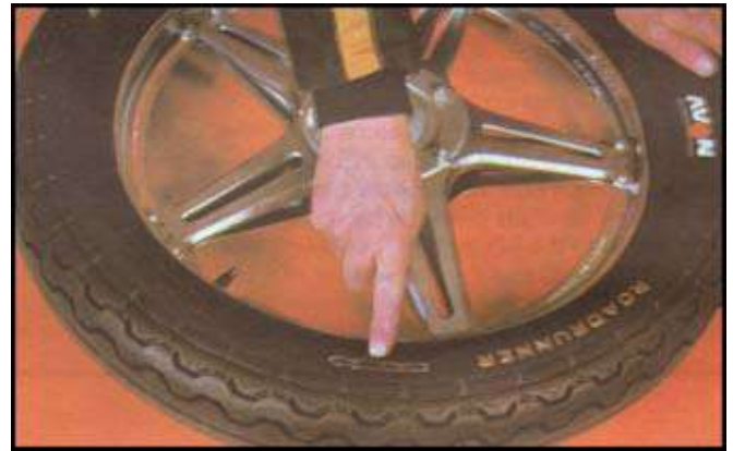
Tyre fitting: Replace first bead over rim noting arrow indicating correct direction of rotation
