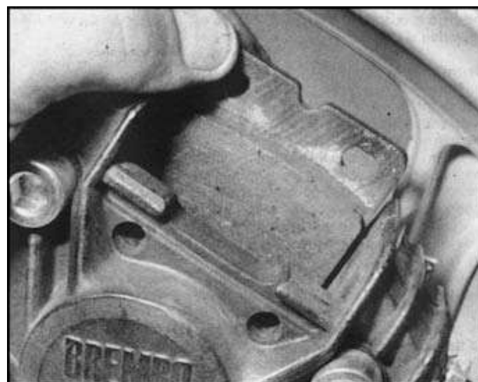
Ensure friction material is against disc when refitting brake pads...
