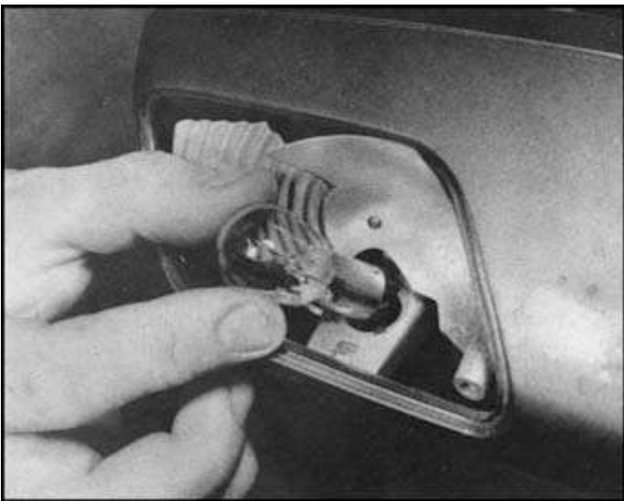
22.16b Bulbs are of bayonet type — press in and twist anticlockwise to release
