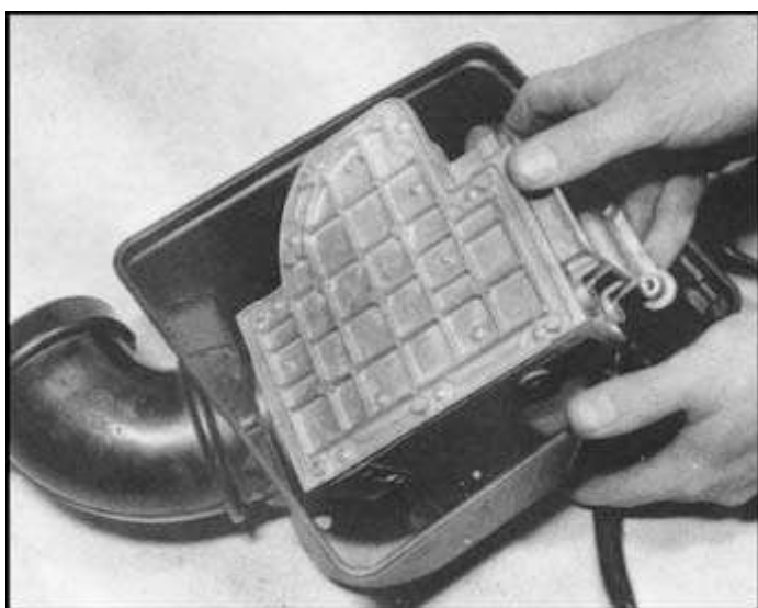
14.6b then slacken hose clamp to release airflow meter
