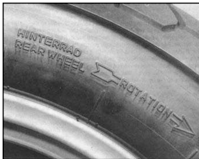
11.7b Arrows on tyre sidewall indicate direction of rotation — see text
