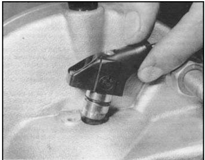
Speedometer impulse transmitter must be removed at regular intervals for cleaning
