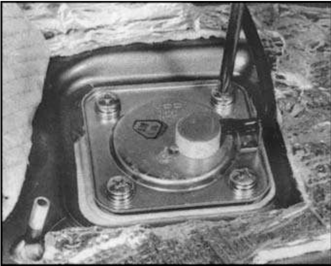
7.4 Fuel gauge sender unit is mounted in underside of tank — later type shown
