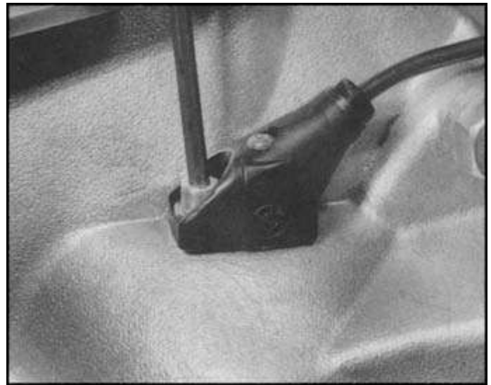
2.2 Speedometer impulse transmitter is retained by a single screw
