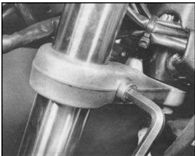
2.5b ... then slacken pinch bolts to release fork stanchions
